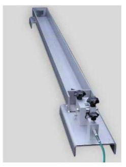
The Shrinkage Drain (1) made of a 1m long u-shaped stainless steel profile which contains the specimen. To avoid wall friction the drain is covered with a removable Neopren ® sheet. On one side a removable anchor is fixed. On the other side this anchor is movable and sliding on three wheels. The motion of this anchor is
